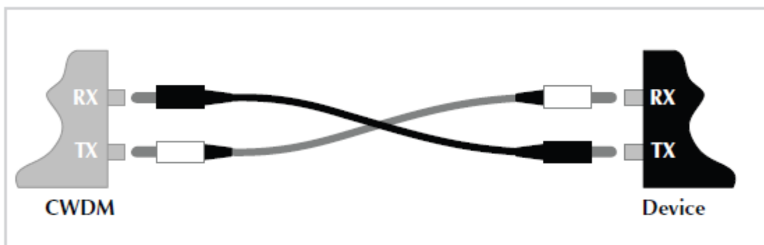
Figure 7: Fiber Cable Connections
